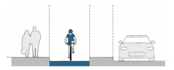
Figure 1. Grade-separated cycle lane
